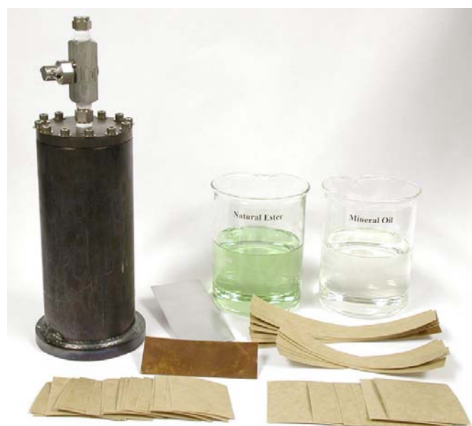
Fig. 1. Components of a sealed test system.
