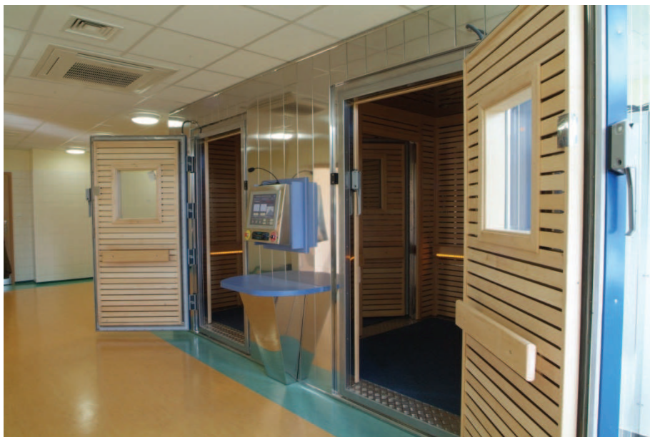
Fig. 3. Two stage cryochamber (CREATOR Sp. z o.o., Poland)
