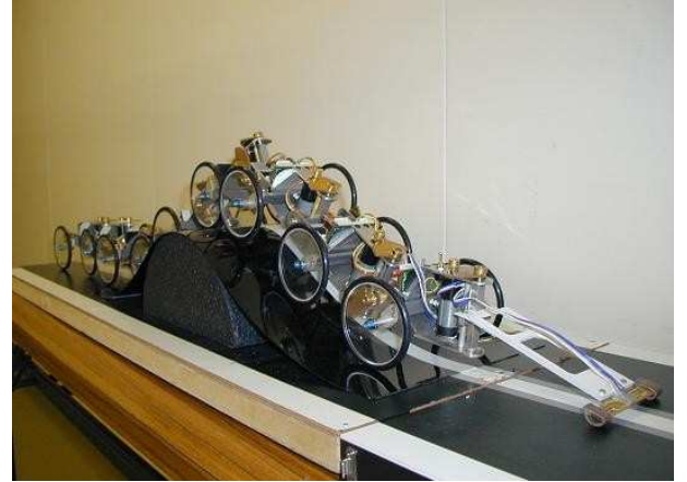
Figure 3. Overview of 9-link locomotive mechanism
