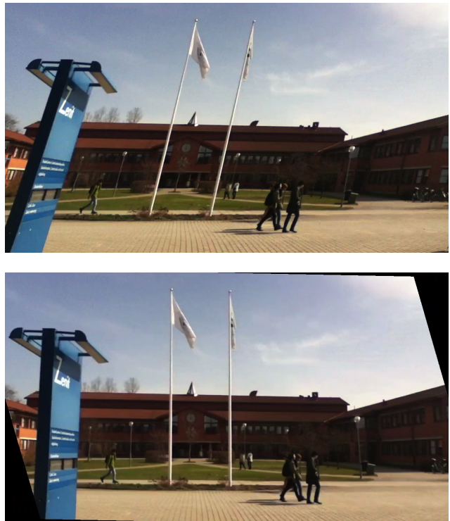
Figure 1. An example of rolling-shutter distortion. Top: Frame from a video sequence recorded with an iPod touch. Bottom: Rectification using the 3D rotation model and inertial measurements.
