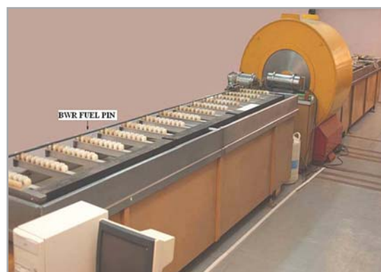
Fig. 1: Gamma Scanner at Advanced Fuel Fabrication Facility, BARC, Tarapur loaded with a BWR fuel pin
