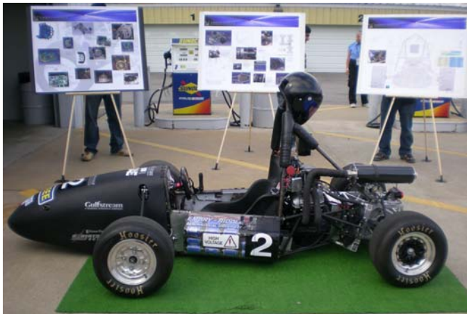
Figure 7: Formula Hybrid Vehicle with Ultracapacitor Banks
