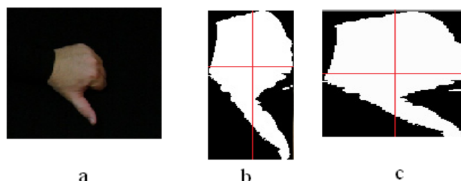
Figure 9. applying trimming process on the input image, followed by scaling normalization process [5].
