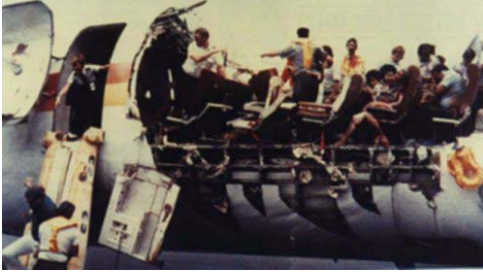
Figure 1 Aloha Airlines Boeing 737-297, registration N73711, operating flight AQ243 from Hilo to Honolulu at Kahului Airport on April 28, 1988 after its fuselage was torn away during flight [1].
