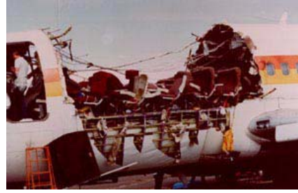
Figure 1 Aloha Airlines Boeing 737-297, registration N73711, operating flight AQ243 from Hilo to Honolulu at Kahului Airport on April 28, 1988 after its fuselage was torn away during flight [1].
