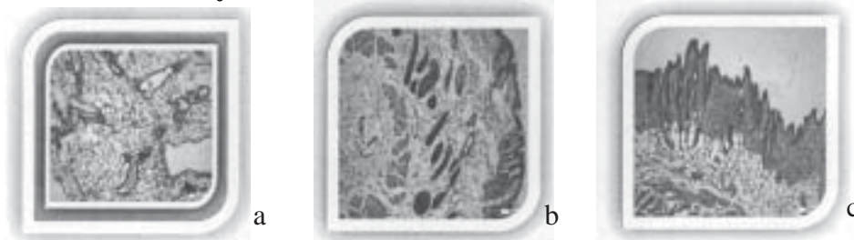
Fig. 2. CoCrMo commercial alloy implanted: a) subjacent area; b) superjacent area; c) lateral area
