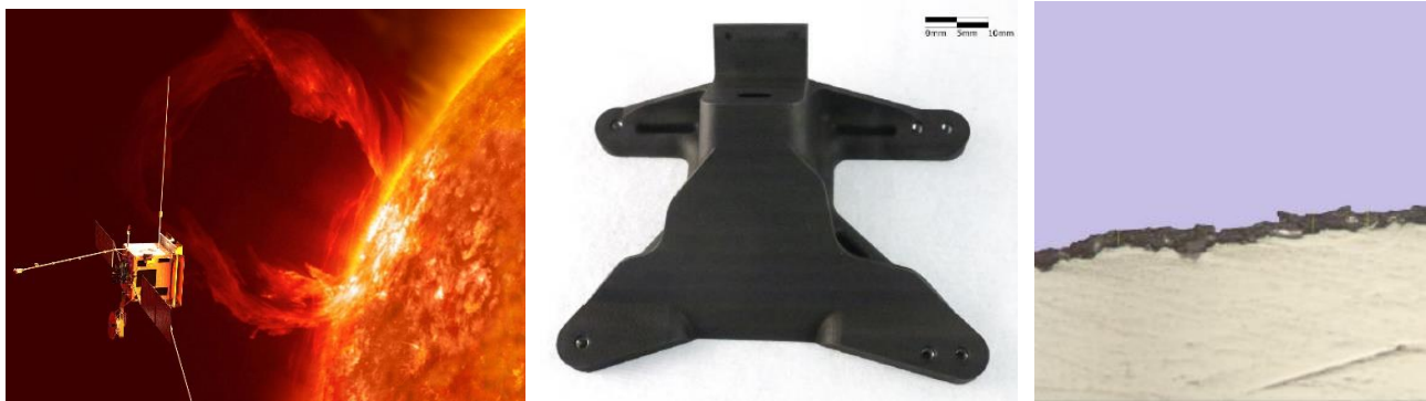
Figure 39 From left to right: The Solar Orbiter Spacecraft (source: esa.int) The Solar black thermal coating on a component of the Solar Orbiter and micro-image of surface layer thickness at 7.8 \mu\text{m} \pm 1.6 \mu\text{m} (source: ENBIO-GSTP ESA workshop presentation)
