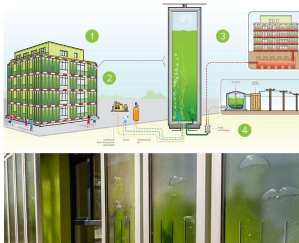
Figure 3 The German developed Bio Intelligent Quotient (B.I.Q.) building system is an example, where live algae farm was used inside the apartments' window façade contributing to its passive energy system. (Wallis, 2013) The algae vertical farm contributes to energy saving system by shading the building, abating street noise and gets harvest to create biofuel and produce heat. (Source: sierraclub.org)
