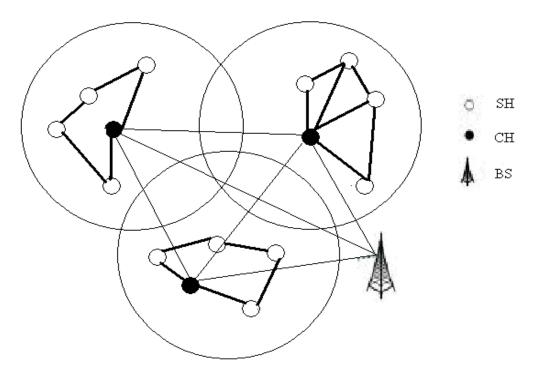
Fig. 1 Clustering in wireless sensor network
