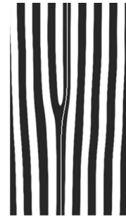
Fig. 1. Inverse Fourier transform of an HRTEM micrograph of STO irradiated crystal showing a series of bent channels in the vicinity of dislocation and the arctan function fitted to the bent channel.
