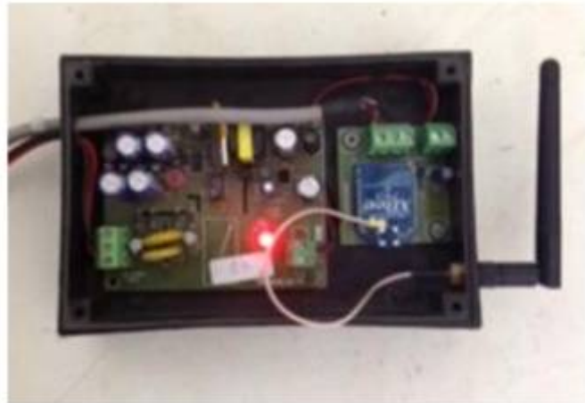
Fig.9. Transceiver unit to interface with base station
