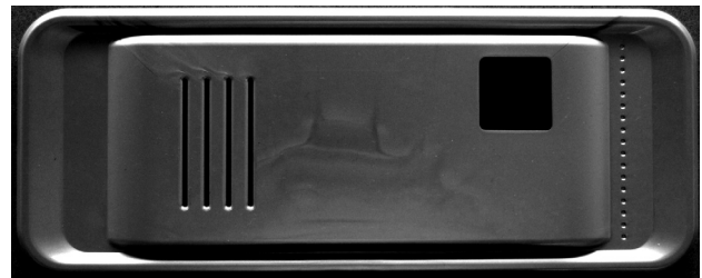
Fig. 4 Real image of injection molded test geometry
