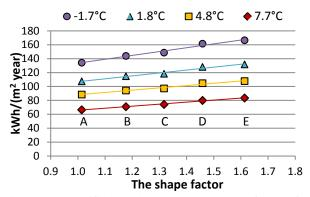
Fig. 2: The specific heat demand vs. the shape factor of the five buildings with thermal envelope scenario called <u>Low</u> in Table 2, and different annual average outdoor temperatures. The characters 'A' to 'E' signify the case study buildings listed in Table 1.
