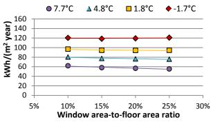
Fig. 8: The effect of the relative window size on the specific heat demand of buildings with <u>Medium</u> thermal envelope scenarios and different climate scenarios.
