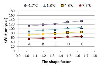
Fig. 3: The specific heat demand vs. the shape factor of the five buildings with thermal envelope scenario called <u>Medium</u> in Table 2, and different annual average outdoor temperatures. The characters 'A' to 'E' signify the case study buildings listed in Table 1.
