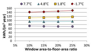
Fig. 7: The effect of the relative window size on the specific heat demand of buildings with <u>Low</u> thermal envelope scenarios and different climate scenarios.
