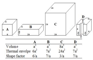
Fig. 1: The shape factor of buildings with different sizes and shapes. The parameter 'a' symbolizes a unit of length.
