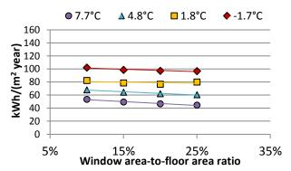
Fig. 9: The effect of the relative window size on the specific heat demand of buildings with <u>high</u> thermal envelope scenarios and different climate scenarios.
