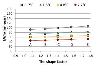
Fig. 4: The specific heat demand vs. the shape factor of the five buildings with thermal envelope scenario called <u>High</u> in Table 2, and different annual average outdoor temperatures. The characters 'A' to 'E' signify the case study buildings listed in Table 1.
