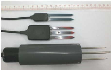
Figure 12: Different types of frequency domain reflectometry sensors which are used in the columnar test.
