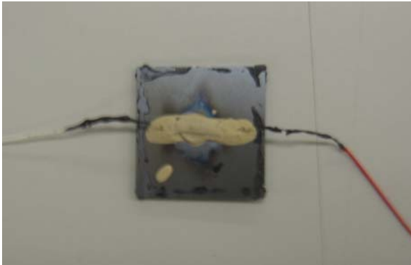
Figure 2 Details of test plate and thermocouple
