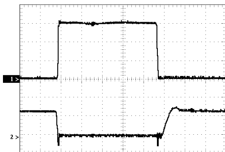
Fig. 5: 1> S1 Drain-Source Voltage (50V/div); 2> S1 Gate-Source Voltage (10V/div) - 1 \mu s/div.
