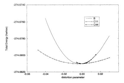
FIG. 7. HF elastic constants. HF total energies for bulk modulus C11 and C44 as a function of the fractional distortion parameter.
