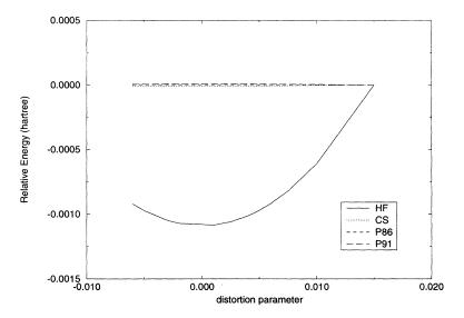
FIG. 6. C44: HF and correlation corrections. Relative energies as a function of the fractional distortion of the lattice corresponding to C44 (relative a = 4.205 Å). Solid line is HF data and dashed lines are correlation-only values. All curves have been zeroed at d = 0.015.
