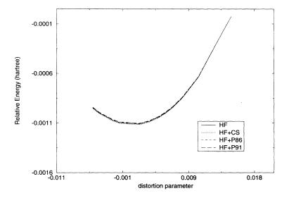
FIG. 5. C44. Relative energies as a function of the fractional distortion of the lattice corresponding to C44 (relative a=4.205 Å). Solid line is HF data and dashed lines include correlation corrections. All curves have been zeroed at d=0.015.
