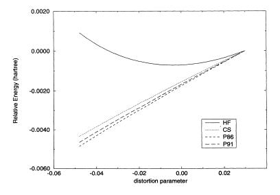
FIG. 4. C11: HF and correlation corrections. Relative energies as a function of the fractional distortion of the lattice corresponding to C11 (relative a = 4.205 Å). Solid line is HF data and dashed lines are correlation-only values. All curves have been zeroed at d = 0.02.
