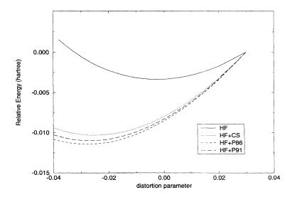
FIG. 1. Bulk modulus. Relative energies as a function of the fractional distortion (d) of the lattice parameter (relative a=4.205 Å). Solid line is HF data and dashed lines include correlation corrections. All curves have been zeroed at d=0.03.
