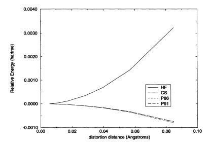
FIG. 10. X-point TO mode: HF and correlation corrections. Relative HF (solid line) and correlation-only (dashed lines) energies as a function of distortion distance from equilibrium (a = 4.205 Å).
