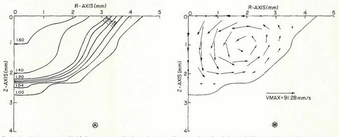
Fig. 6 — Results for run no. 8 of Table 2: A — computed isotherms for run no. 8 representing a sharply focused 190 A arc without surface tension driven flow taken into account. B — computed velocity map
