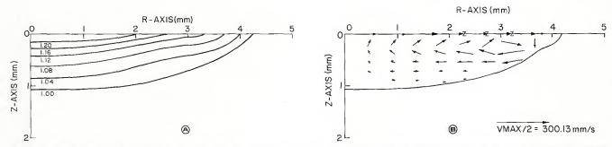
Fig. 3 – Results for run no. 2 of Table 2: A – computed isotherms for run no. 2, representing a broadly focused 100 A arc. B – computed velocity map
