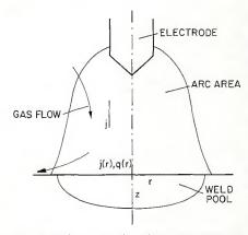
Fig. 1-Schematic of welding arc showing relative size of weld pool, electrode and arc
