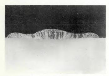
Fig. 7 – Profile of a stationary weld made for 3 s at 235 A on Type 304 stainless steel plate; compare this actual profile with the shape of the computed isotherms shown in Fig. 4A
