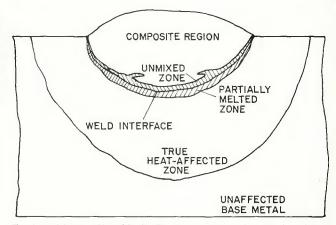
Fig. 8 – Mixing profile of high alloy Type 310 stainless steel on lower alloy Type 304 stainless steel base metal as measured by Savage et al. (Ref. 7). Note the protrusions of unmixed but fused base metal suggesting the presence of stagnation points in the velocity profile
