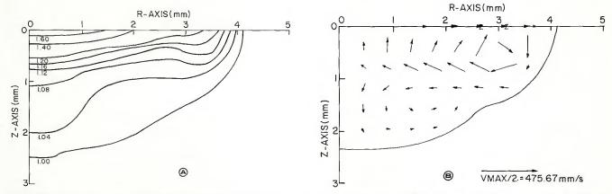
Fig. 4—Results for run no. 3 of Table 2: A—computed isotherms for run no. 3 representing a sharply focused 190 A arc. B—computed velocity map
