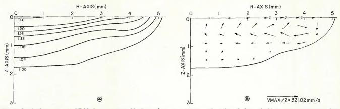
Fig. 5—Results for run no. 4 of Table 2: A—computed isotherms for run no. 4 representing a broadly focused 190 A arc. B—computed velocity map
