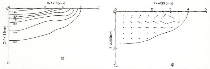
Fig. 2 – Results for run no. 1 of Table 2: A – computed isotherms expressed as a fraction of the absolute melting temperature for a stationary weld with the parameters of run no. 1; this represents a sharply focused 100 A arc. B – computed velocity map
