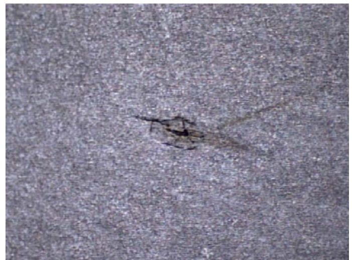
Figure 5. Small Base Metal Flaw as Magnified (PVRUF)
