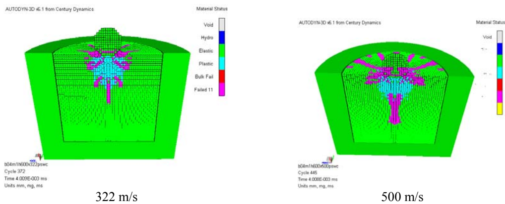
Figure 5. Results at 4 \mu s for B = 0.4 , M = 1.0 . 600 MPa tensile strength for WC sphere.
