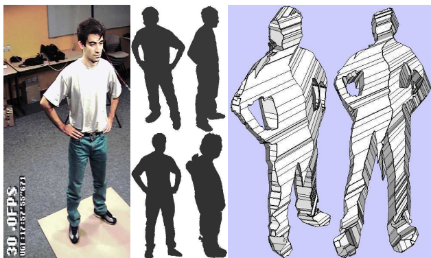
Figure 1: Real time reconstruction of a real person with 4 cameras.
