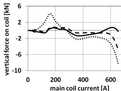
Figure 8: Measured total vertical force on the main coil. Dotted line= during the initial ramp-up, dashed line= after vertical positioning of the main coil and full line= after application of all shims on the top yoke.
