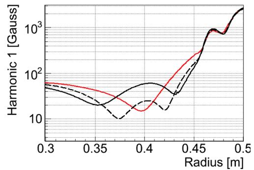
Figure 4: First harmonic component in the field map: red full line= measured with a slightly horizontally displaced main coil, black full line= measured with a horizontally centered main coil, black dashed line= calculated first harmonic from the OPERA3D field map.
