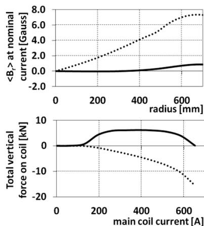
Figure 6: (top) calculated average radial fields in the S2C2 with (full line) and without (dotted line) shims on the top yoke. (bottom) calculated total vertical force on the main coil with and without shims.
