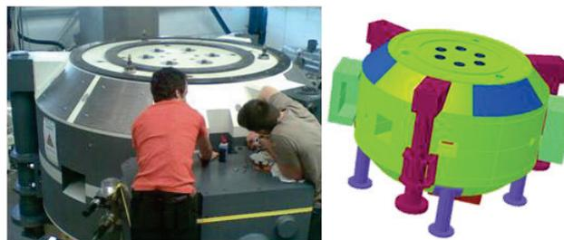
Figure 7: (left) shims applied on the S2C2 (may 2013) (right) OPERA3D model of the S2C2 with all shims included on the top yoke.
