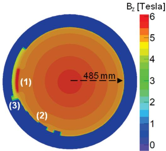
Figure 2: Full measured field map of the S2C2 at nominal current. (1) = the regenerator region, (2) = limited radial range due to presence of the septum in the median plane and (3) entrance of the extraction channel.
