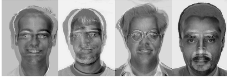
Fig. 1. Common Vectors corresponding to 4 of the classes in the AR dataset used.
