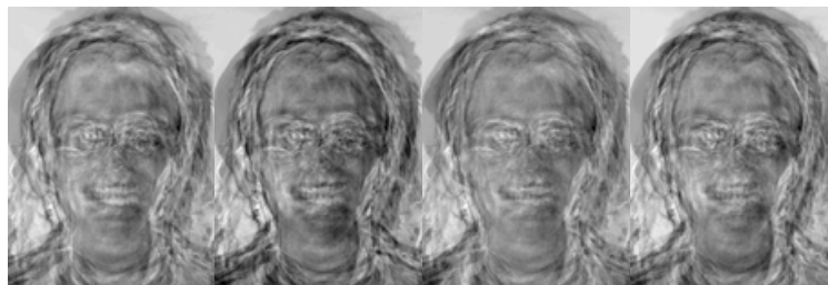
Fig. 2. Discriminant Common Vectors corresponding to 4 of the classes in the AR dataset used.
