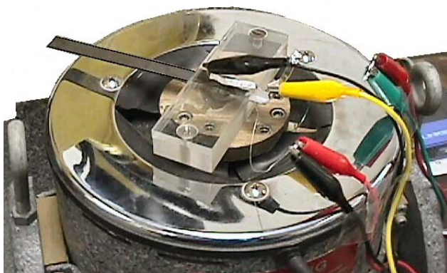
Fig.6 A hybrid beam mounted on a shaker.
