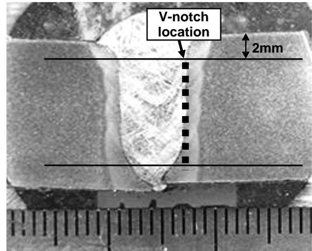
Fig. 10 Machining position of CVN specimen and V notch location.
