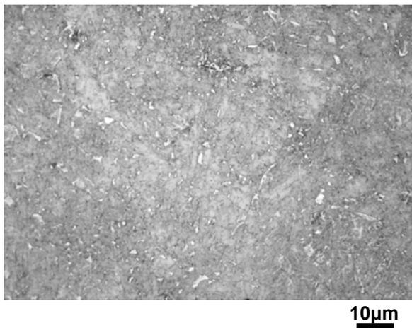
Fig.12 Optical micrographs of mid-wall of quenched pipe with 40 mm WT (Le Pera's etching).
