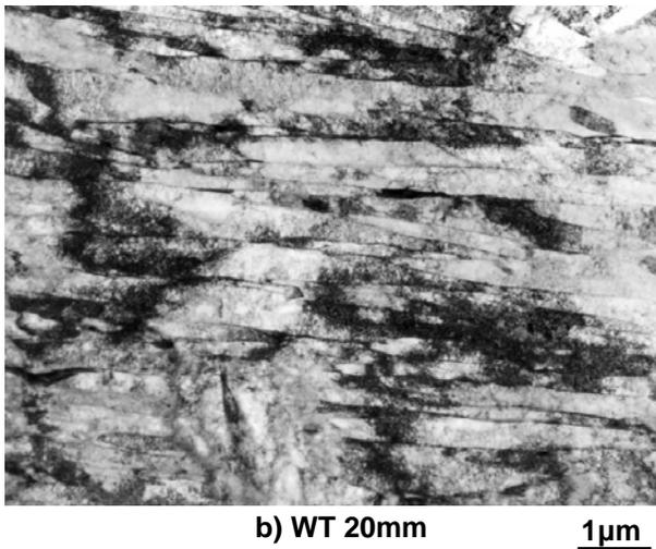
Fig.11 TEM images of mid-wall of quenched pipes.
