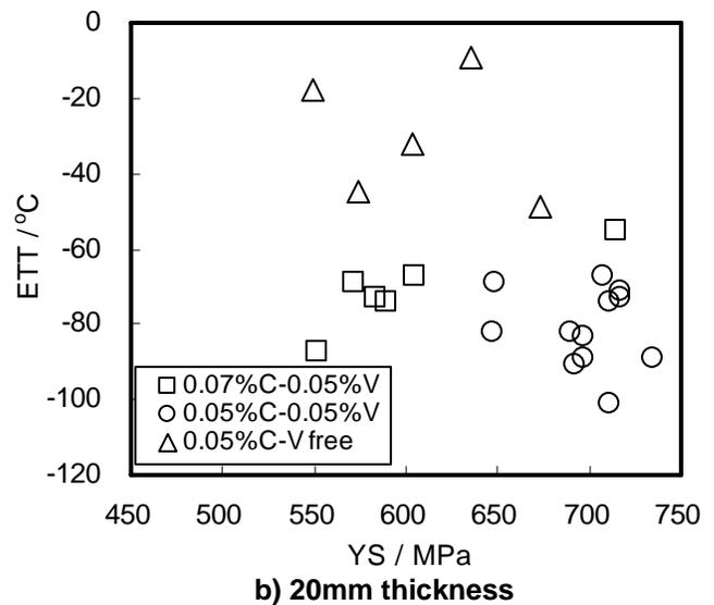
Fig. 5 Relationship between yield strength (YS) and energy transition temperature (ETT) of simulated inline QT steel plate (CVN test of T-direction).
