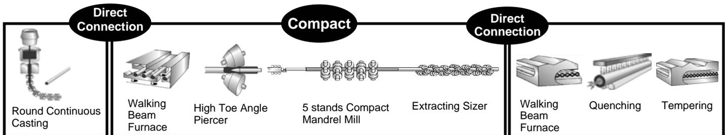
Fig. 1 Schematic illustration of the newly-constructed medium size mill and inline heat treatment facilities.
