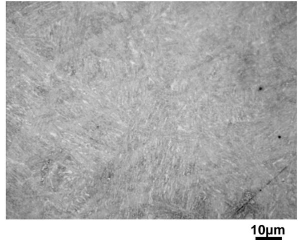
Fig.13 Optical micrographs of mid-wall of quenched pipes with 20mm WT (Le Pera's etching).
