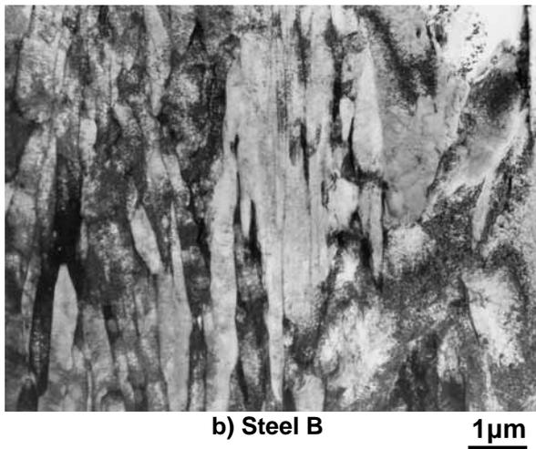
Fig. 6 TEM image of quenched steel plate (mid-thickness portion of wall thickness 40mm).
