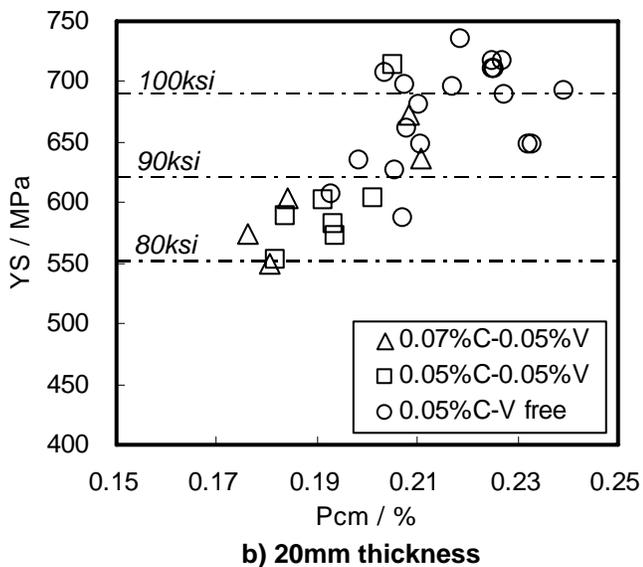
Fig. 4 Effect of Pcm on yield strength of simulated inline QT steel plate (tensile test of L-direction).
