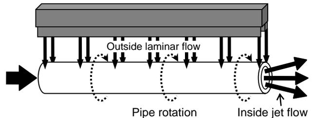
Fig. 2 Schematic illustration of the quenching device.
