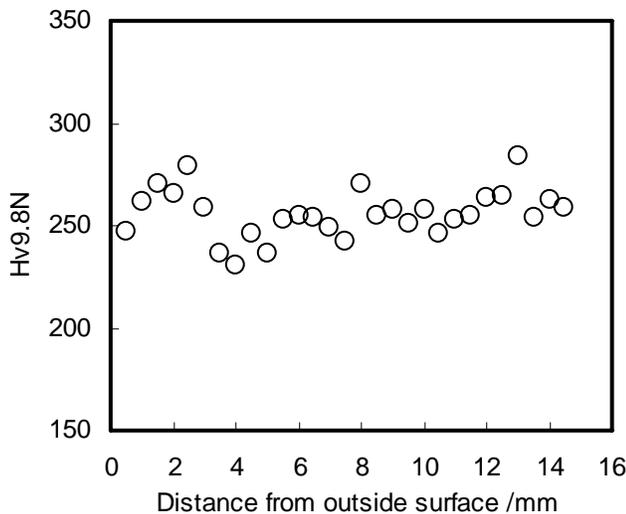
Fig. 9 Hardness distribution along fusion line of welding test.
