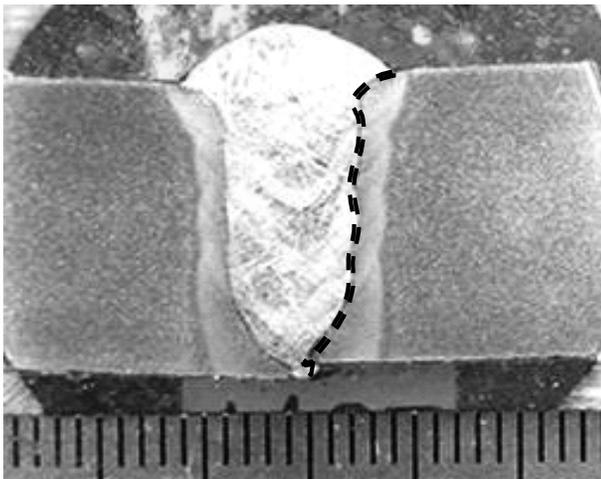
Fig. 8 Typical macrostructure of welding portion and location of hardness measurement.
