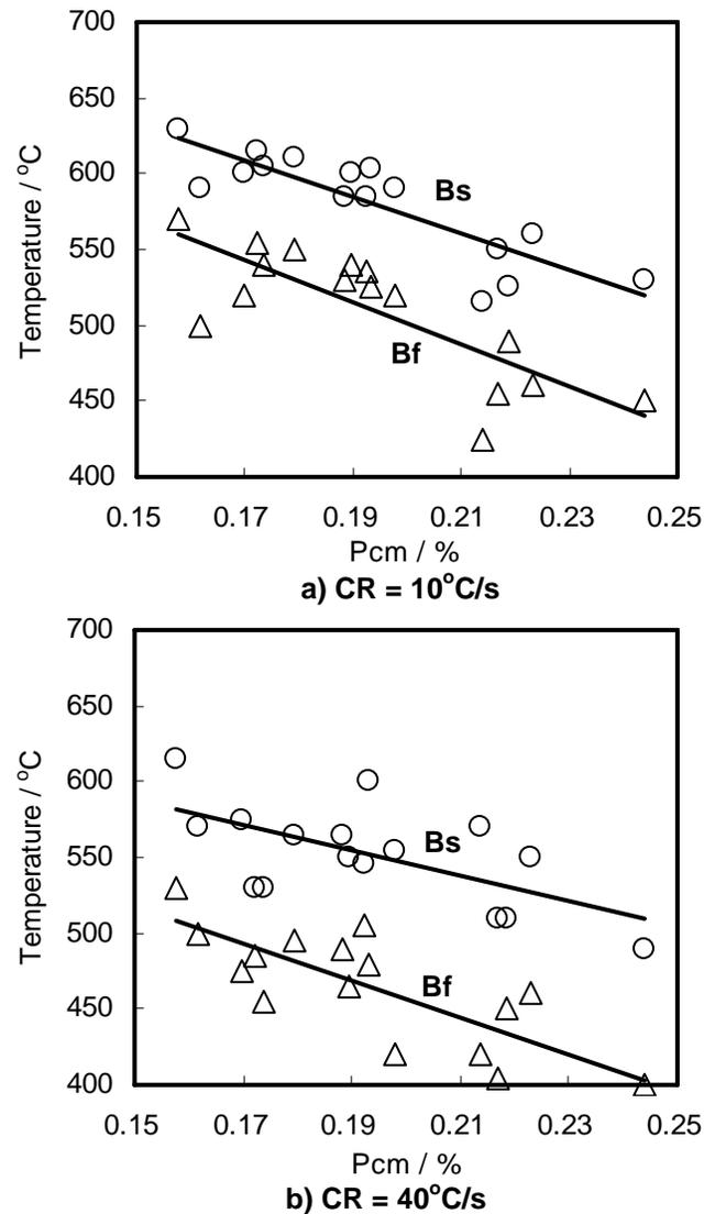
Fig. 3 Effect of Pcm on transformation temperature during continuous cooling from austenite phase (thermodilatometry test).
