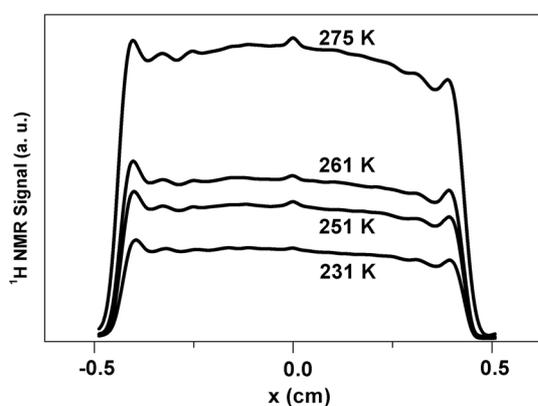
Fig. 1c. Examples of 1D profiles of the water protons confined in pores of white cement as functions of temperature.
