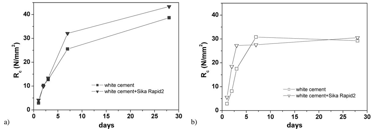
Fig. 5. Compressive strength development of (a) white cement, sample *Wa* (solid squares) and white cement with Sika Rapid 2, sample *Wb* (solid triangles) and (b) white cement, sample *Da* (open squares) and white cement with Sika Rapid 2, sample *Db* (open triangles). The samples were hydrated in constant wet (*samples W*) and dry (*samples D*) conditions, respectively.
