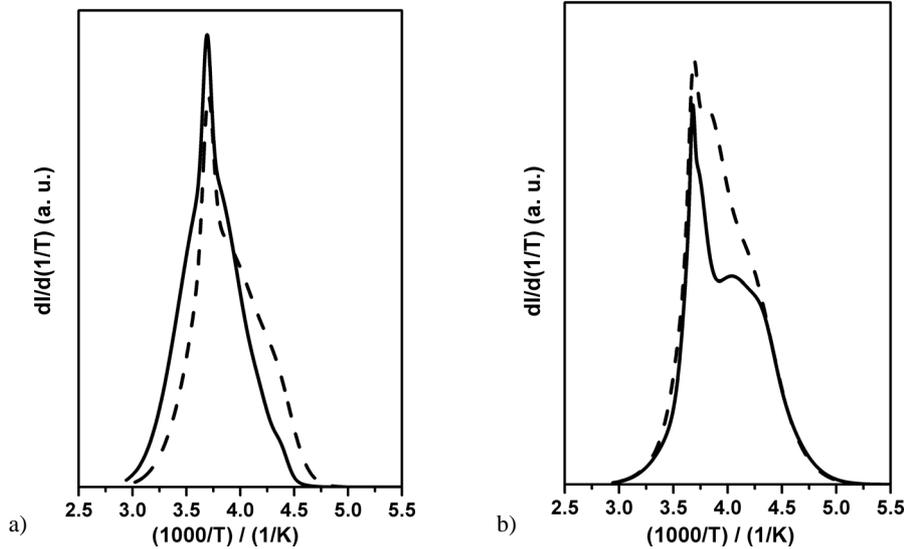
Fig. 3. Melting point distribution curves derived from (8) for water confined in pores of (a) white cement, sample *Wa* (solid line) and white cement with Sika Rapid 2, sample *Wb* (dashed line) and (b) white cement, sample *Da* (solid line) and white cement with Sika Rapid 2, sample *Db* (dashed line). The samples were hydrated in constant wet (*samples W*) and dry (*samples D*) conditions, respectively.
