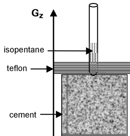
Fig. 1a. The setting of the probe for the  $^1\text{H}$  NMR measurements in the one-dimensional  $^1\text{H}$  Single Point Imaging (1D  $^1\text{H}$  SPI) measurements, showing also the direction of the applied gradient  $G_z$ .
