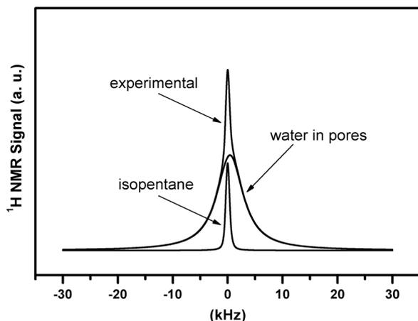
Fig. 1b. Examples of the spectrum obtained for water protons confined in pores of white cement at 251 K. Also the signal from isopentane, which serves as the calibration signal, is seen.
