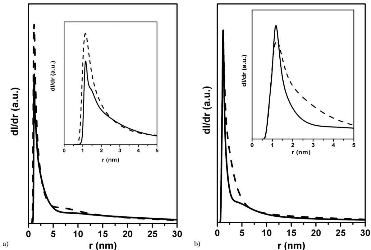
Fig. 4. Pore size distribution curves derived from (9) for water confined in pores of (a) white cement, sample *Wa* (solid line) and white cement with Sika Rapid 2, sample *Wb* (dashed line) and (b) white cement, sample *Da* (solid line) and white cement with Sika Rapid 2, sample *Db* (dashed line). The inset shows the distribution of smaller pores for the samples. The samples were hydrated in constant wet (*samples W*) and dry (*samples D*) conditions, respectively.
