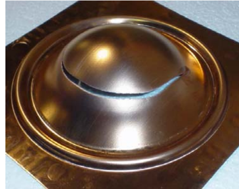
Figure 5. Experimental result of forming of 99.9% copper sheet.
