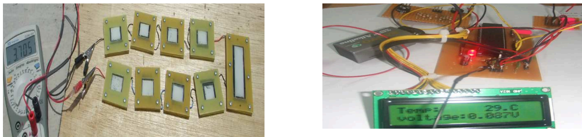
Fig.2: Design of DSSC housing and circuit to measure the voltage and temperature
