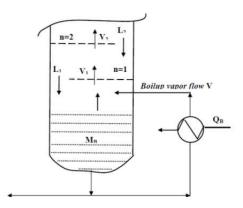
Fig. 3.4. Bottom Section and Re-boiler
