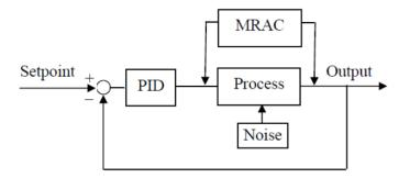
Fig. 6.2. Adaptive controller with MRAC and PID
