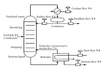
Fig. 2.1. Control Valves Location
