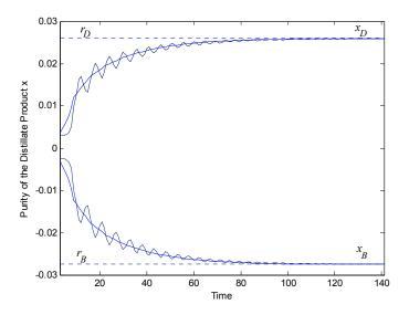
Fig. 6.3. Correlation of Plant Outputs, Model Outputs and Reference Setpoints
