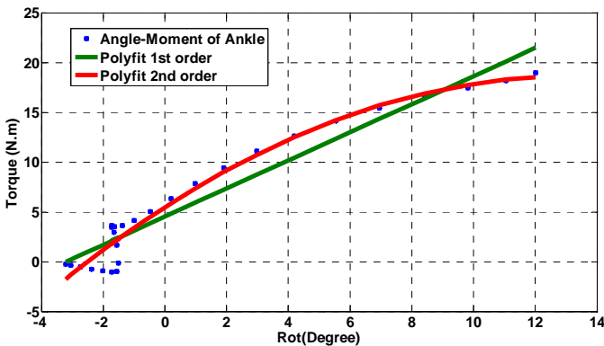
FIGURE 4: ANKLE TORQUE VS. ROTATION FOR SLOW WALKING SPEED IN SWING PHASE OF THE GAIT
