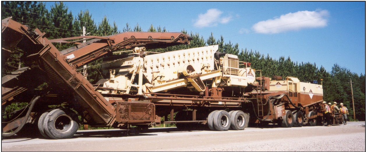
Figure 2. Cold-In-Place Recycling Train
