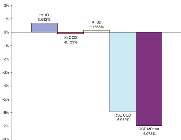
Figure 7. Predictions using various techniques for  $\sigma_1$  95% quantile in percent difference compared to 800 LHS runs
