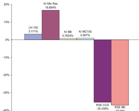
Figure 8. Predictions using various techniques for  $\sigma_2$  95% quantile in percent difference compared to 800 LHS runs
