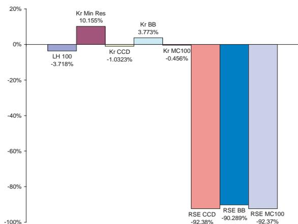
Figure 6. Predictions using various techniques for  $T_1$  standard deviation in percent difference compared to 800 LHS runs
