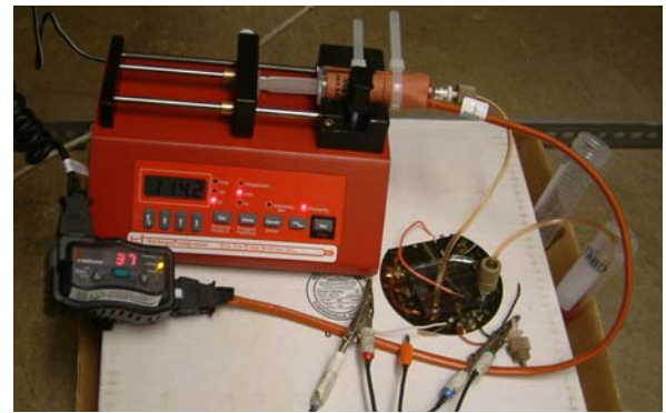
Fig. 9: The experimental setup for electrical impedance measurement of blood rheological parameters.
