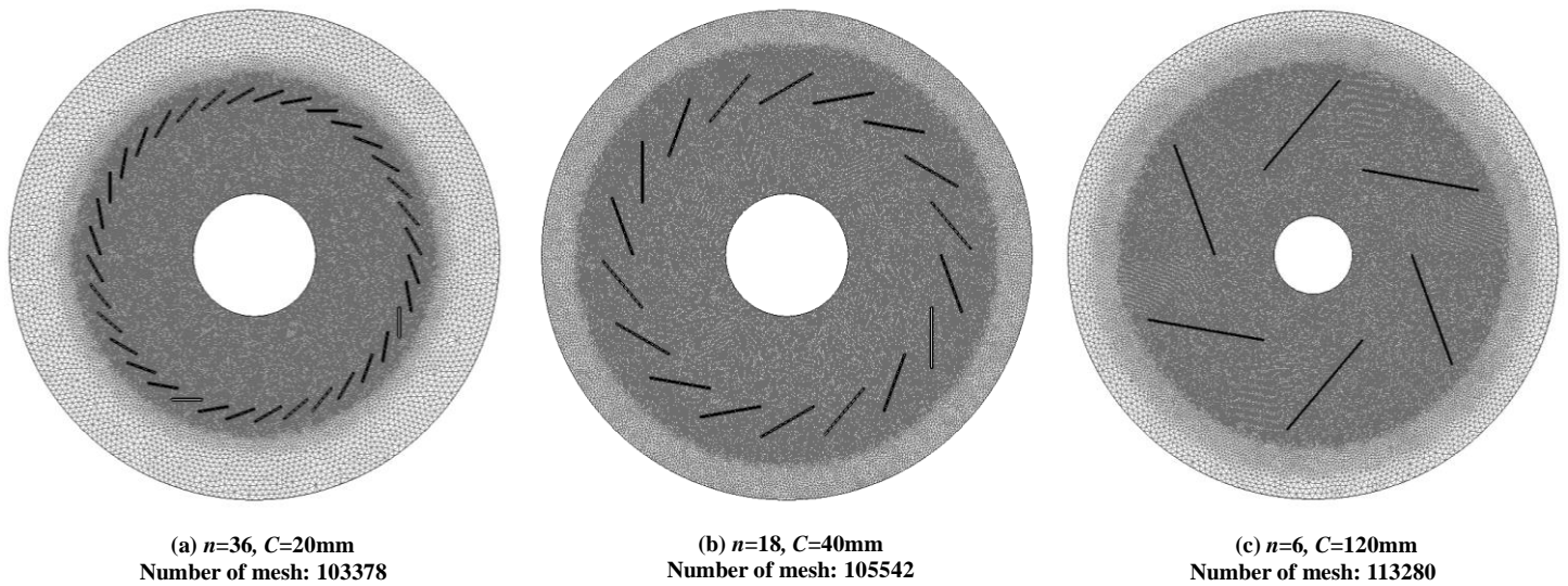
Figure 2. Typical calculation mesh for various numbers of vanes and identical solidity ( r_3/r_2=0.4 , \beta_2=20\text{deg} , s=1.14 )
