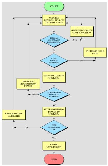
Fig. 3 SPV Algorithm flowchart.
