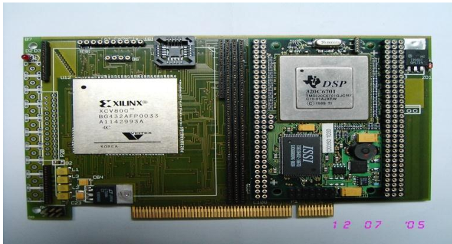
Fig.8 Universal Digital signal processor Data Acquisition board (UNIDAQ)
