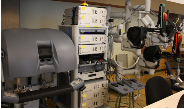
Fig. 7. Research da Vinci System at UBC, with 6 controller boxes (and 1 spare) to power 2 MTMs, 3 PSMs, and 1 ECM (functionally compatible with a PSM). Photo courtesy of Omid Mohareri, UBC.
