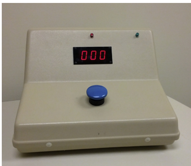
Fig. 1. The Gordon Diagnostic System has an LED display upon which stimuli are presented, and a large blue button for making responses. The red and green lights do not provide feedback on performance, but only indicate whether a data collection session is ready to proceed or has terminated. (For interpretation of the references to colour in this figure legend, the reader is referred to the web version of this article.)
