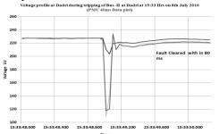
Figure 4 Fault clearing time visualization through PMU
