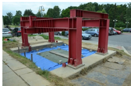
Fig. 1 Heavy steel test frame
