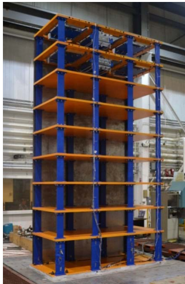
Figure 1. 9 story test structure
