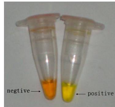
Fig. 3. Detection of loop-mediated isothermal amplification (LAMP) products after addition of SYBR Green I. The solution turned yellow in the presence of LAMP amplification products but remained orange in the absence of the amplicon.
