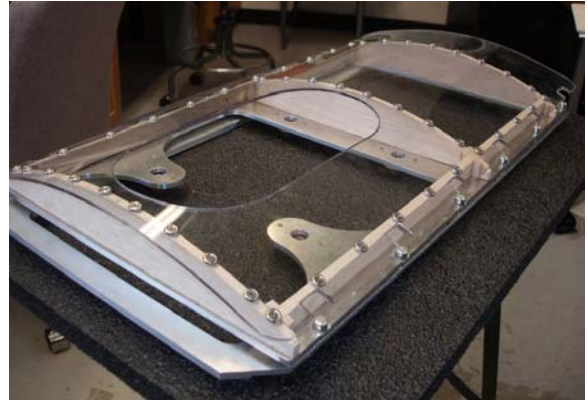
Figure 7. Payload mounting interface bracket.
