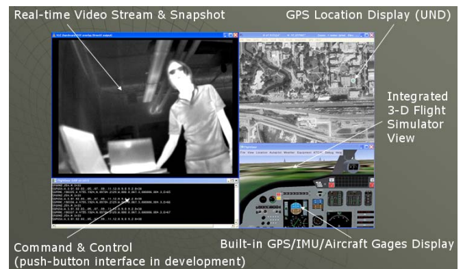
Fig. 5. The ground control station user interface.
