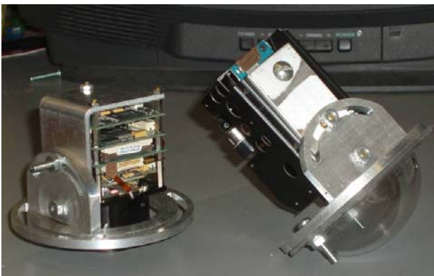
Fig. 6. Custom camera brackets to allow manual pointing.
