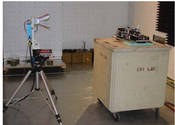
Fig. 8. EMI test setup performed at Lockheed Martin.
