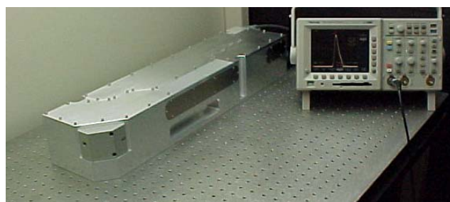
Figure 10: Photograph of next-generation high-power diode-pumped Q-switched intra-cavity frequency-converted 355 nm laser.
