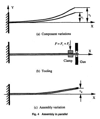
the free ends were joined and  $\nu_{a2}$  which was a fixed end for Beam 2.
