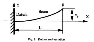
Next, consider two components with variations  $\nu_1$  and  $\nu_2$  at their respective free ends joined mechanically. (The assumption of mechanical joining is made so that later calculations are unencumbered by thermal considerations. In other words, a weld nugget is indistinguishable from a rivet.) The problem is to determine the parameters  $c_i$  in Eq. (3). Two basic configurations are examined.
