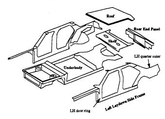
Fig. 1 Automotive body panel structure
