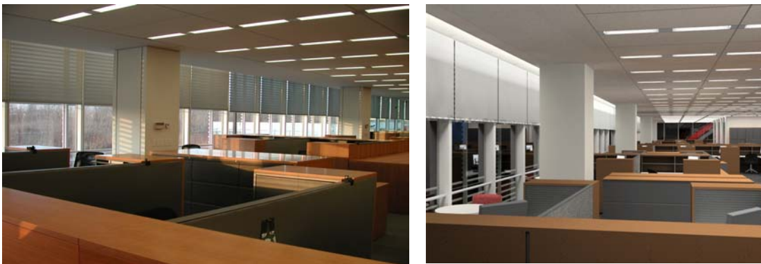
Figure 2. Photograph of mockup (left) and RADIANCE nighttime rendering of the same space (right)
