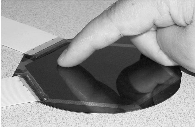
Fig. 2. Photograph of finger on electrode array.
