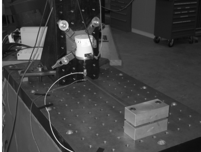
Figure 3.2. The test setup used in the experiments, a cantilever beam. Point acceleration is measured in its free end.
